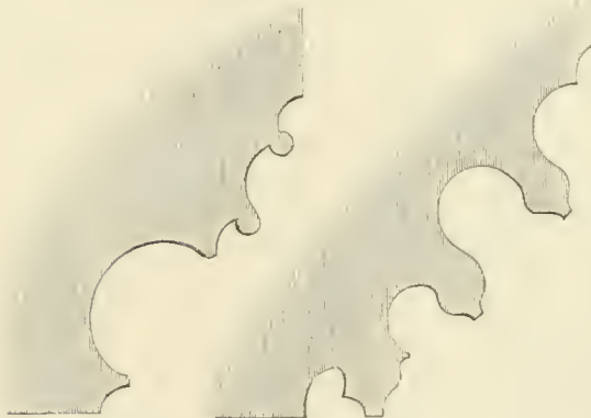
Modern Jamb Mould weak and wiry.
